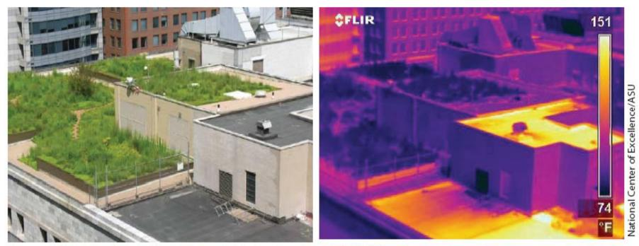
On a typical day, the Chicago City Hall green roof measures almost 80°F (40°C) cooler than the neighboring conventional roof.
