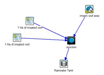
Figure 2 MUSIC model layout showing 2 Ha of irrigated roof with 6 Ha of impervious roof area.
