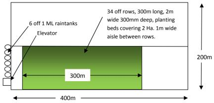
Figure 1 Sketch showing a plan view of the 8 Ha distribution centre (not to scale)
