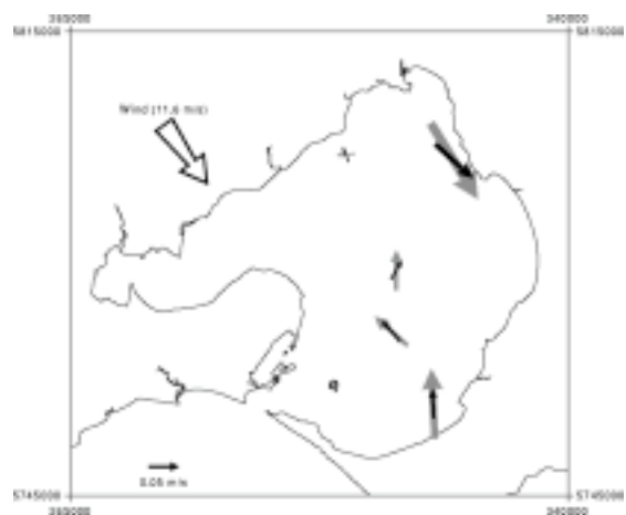
Figure 3 Mean current measured for 17-18 May 1994.
