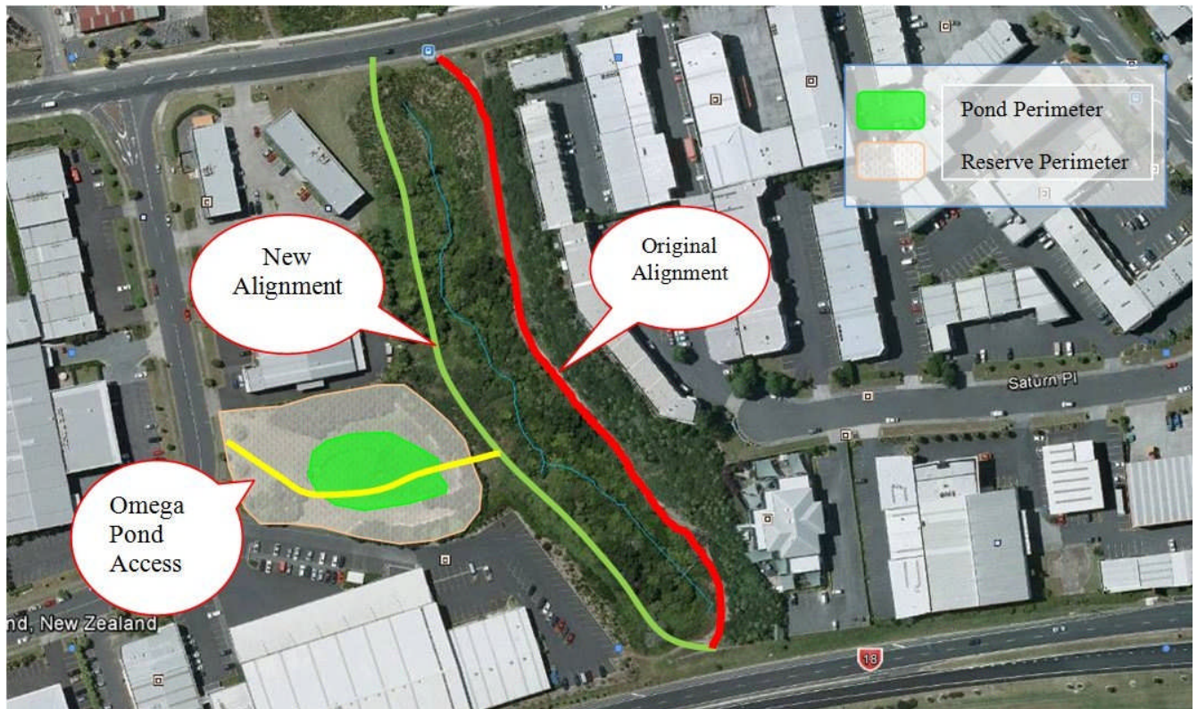
Figure 6: Original cycle-way alignment in red, proposed change in green and access through the Pond in yellow
